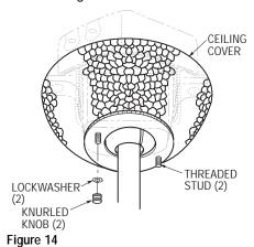
To avoid possible fire or shock, make sure that the electrical wires are completely inside the outlet box and not pinched between the ceiling cover and the ceiling.
